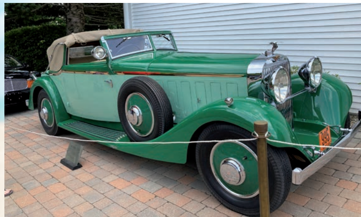
This amazing vehicle is a 1934 Hispano-Suiza sedan from France with an overhead valve V-12 engine that generated 220 horsepower—incredibly advanced for that day!
